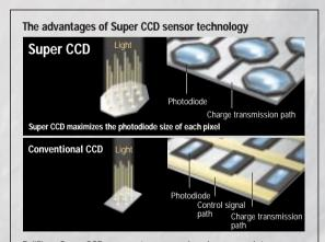
Fujifilm's Super CCD represents a comprehensive approach to improved imaging performance, not only by capturing higher resolutions but also by enhancing each of the other various factors that comprise image quality.
